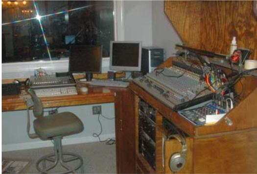
The sound/ control room is isolated as well as sound proof from the stage. A 32 channel snake brings your signal from the stage. The control room is equipped with a 32 track live mixer as well as a 24 track digital recorder (Roland Vs2400Cd studio)
